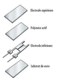
**Principle of capacitive hygrometer:** The sensitive element of a hygrometer is a capacitance whose dielectric is made from a hygroscopic substance. This substance, with a thickness of few micrometers, is a polymer that absorbs water molecules contained in the air. As a result, the capacitance varies. A electronic device converts this capacitance variation into a relative humidity value.
